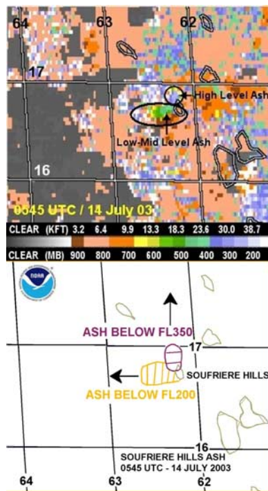
Figure 5. Cloud top height product based on the GOES-12 Imager CO 2 Analysis Technique (COAT) (top) compared with the VAAC analysis both valid 0545 UTC, 14 July 2003.
